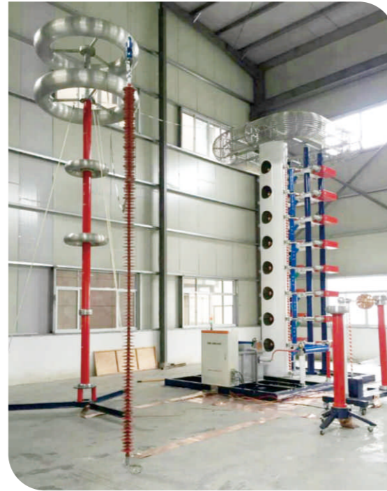
▲ 2800kV 280kJ ▲ 1600kV 45kJ for insulator testing
