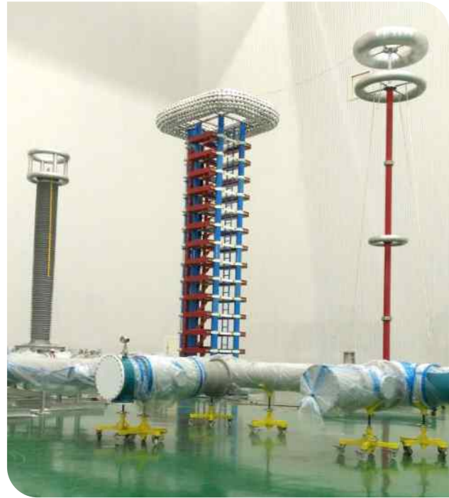
▲ 2800kV 280kJ ▲ 1600kV 45kJ for insulator testing
