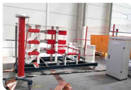
▲ 2800kV 280kJ ▲ 1600kV 45kJ for insulator testing
