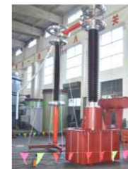
300kV 1A Tank Type Transformer
