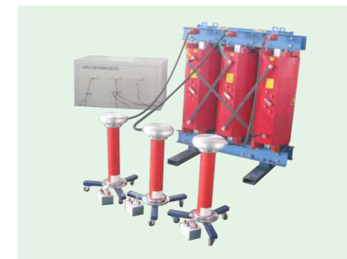
PD Test System For Transformer
