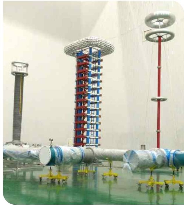
▲ 2800kV 280kJ ▲ 1600kV 45kJ for insulator testing
