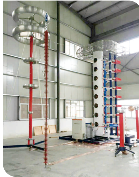
▲ 2800kV 280kJ ▲ 1600kV 45kJ for insulator testing
