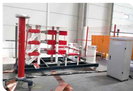
▲ 2800kV 280kJ ▲ 1600kV 45kJ for insulator testing
