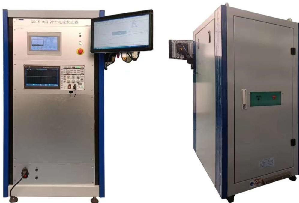
Fig 1 impulse voltage generator without test cabinet for test specimen
