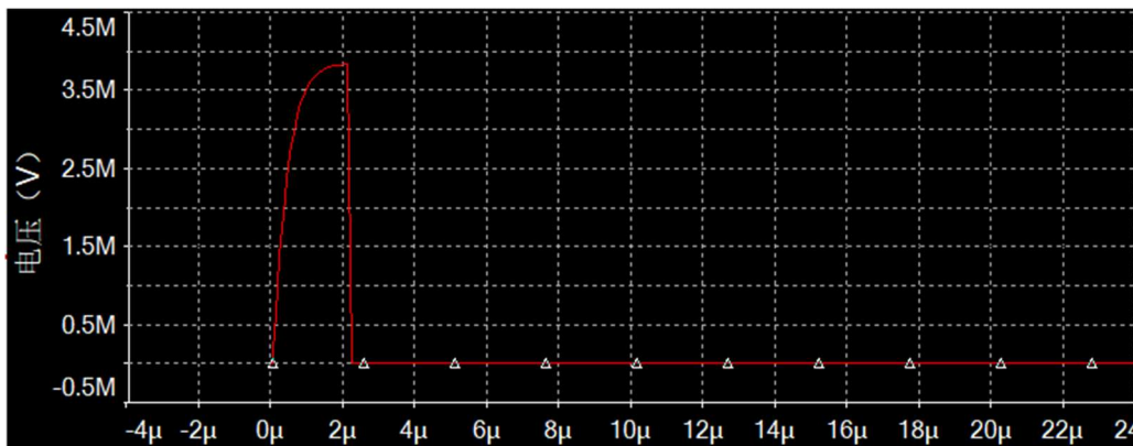
2 \mu s wave generated by 4800kV HV Generator
